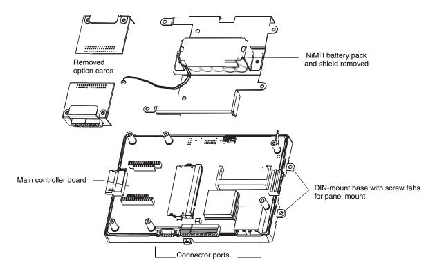
Fig. 2. WEB/CP-700 main controller board and 2 option cards uninstalled.
